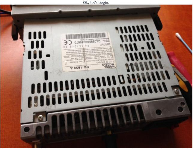
Firstly, remove the headunit from the dash, unscrew the 2 screws that are on the top of the unit and take of the lid.
