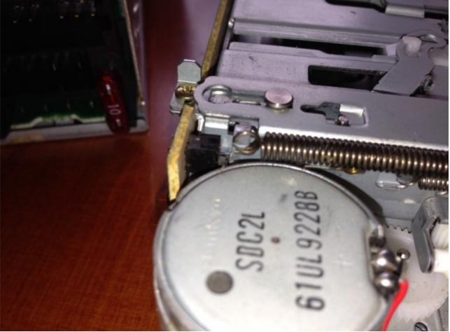
This switch is like a sensor, which tells the headunit whether a cassette is in the headunit or not. You need to unsolder this switch. I used some solder wick for the job:
