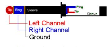
3.5 mm stereo pinout suhastech.com
