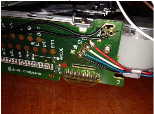
Soldered two wires on the pads where we desoldered the switch:
